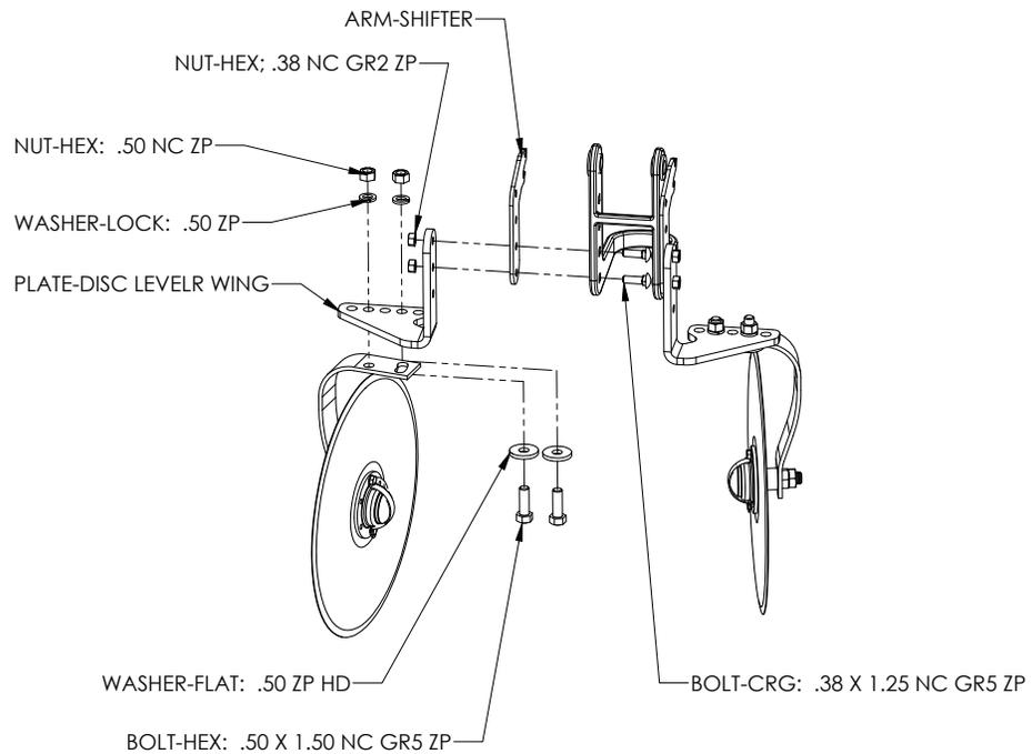
**NOTE:** The disc leveler mounting instructions are only a starting point. The final field adjustment must be made by the operator to achieve the leveling desired. It is recommended that adjustments are made on only three or four levelers, side by side on the outside of a wing. Adjust those levelers until desired leveling is achieved before proceeding to the remaining levelers.
