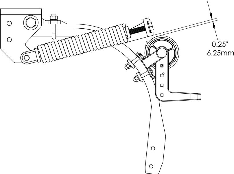
Determine proper arm height and disc width. Disc height should be 1-3" above sweep point depending on planting depth.
