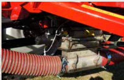
The shut off slide isolates the meter from the tank.
